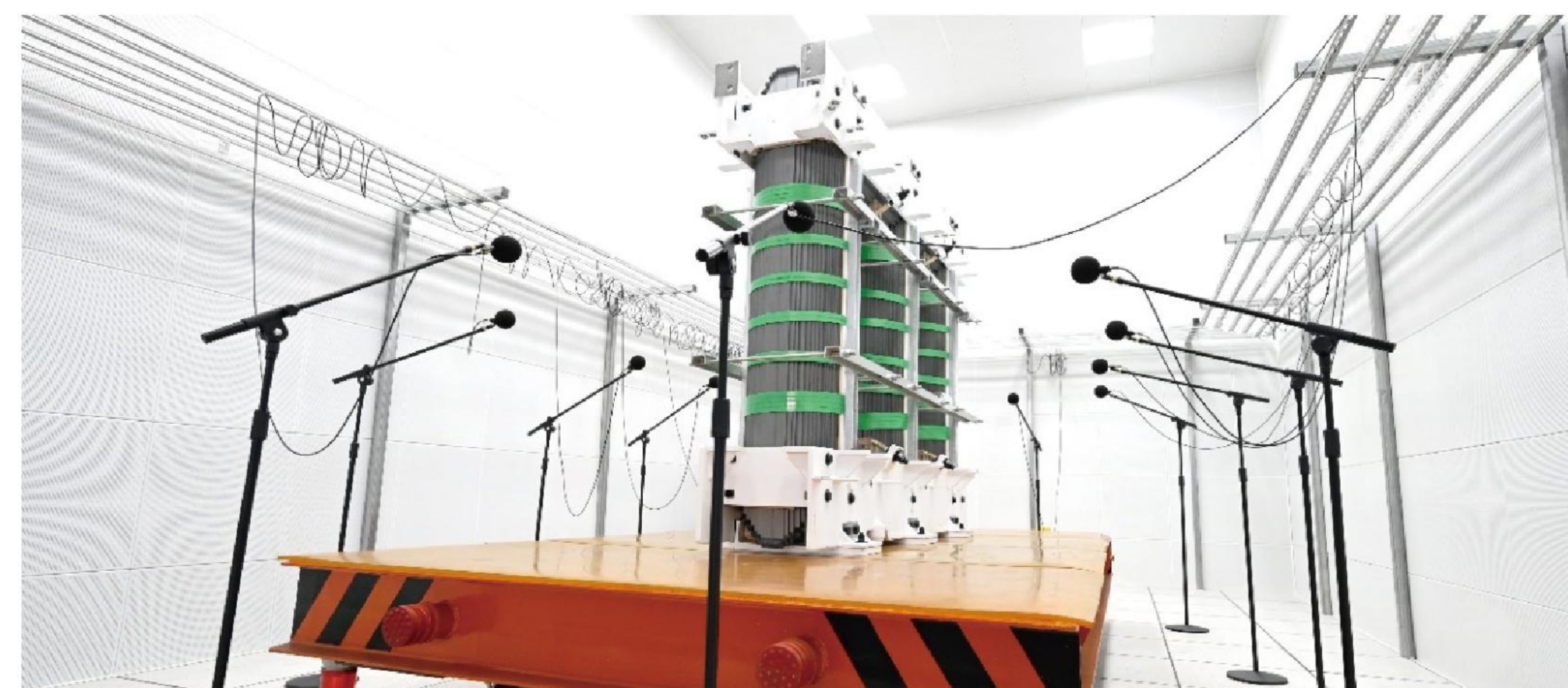
Testing Equipment - Multi-Channel Vibration and Noise Data Acquisition and Analysis System
